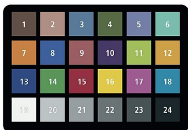
Rys. 2. Wzornik X-rite ColorChecker z zaznaczonymi numerami pól Fig. 2. X-rite ColorChecker with marked number on each color square
